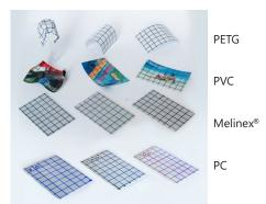
After 5 mins After 5 mins After 5 mins at 150 C at 100 C at 85 C
